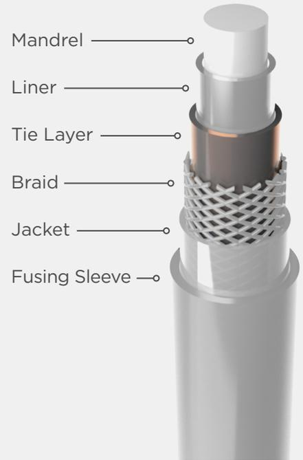
*Tie Layer creates a melt-bondable surface that improves adhesion to both the liner and catheter jacket during the reflow process.*
