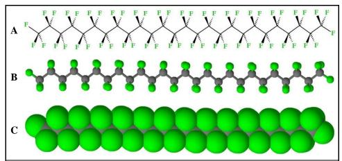
**Figure 3: Structure of PTFE. A)** Stereo bond-line drawing, **B)** ball-and-stick model, and **C)** space-filling model of PTFE (*shown as zig-zag depiction*). (Conformations of PTFE are variable during melt and amorphous phases).
