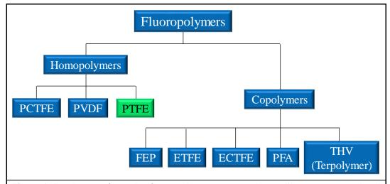
**Figure 1: Landscape of popular fluoropolymers.** Homopolymers like PTFE are produced through the polymerization of identical monomer units. Copolymers incorporate two or more monomers to produce the final polymer material.
