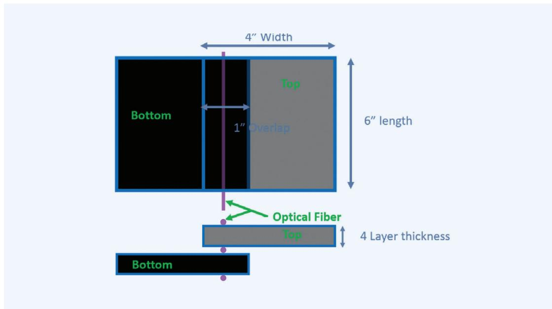
Figure 4. Laminate Welding Configuration
