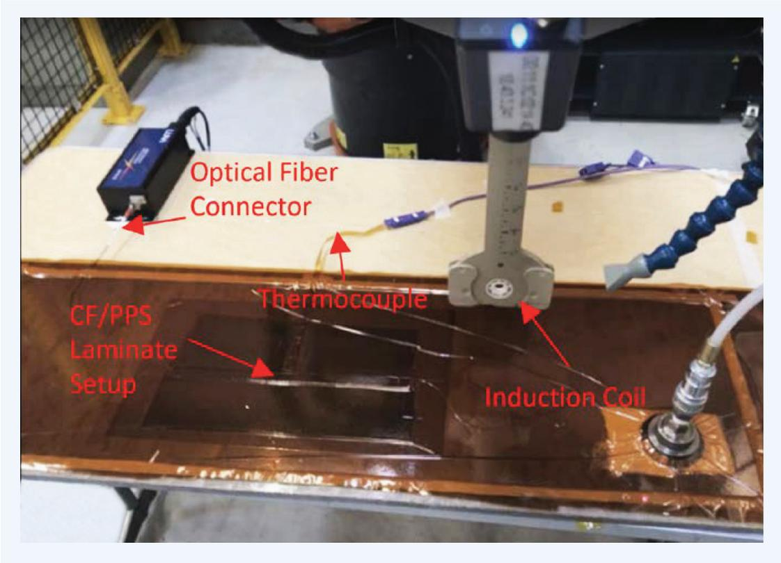
Figure 3. Induction Welding Setup
