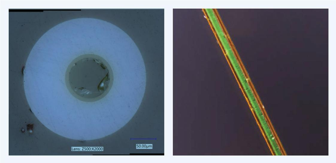
Figure 2. (Left) PPS Coated HD-FOS Sensor
