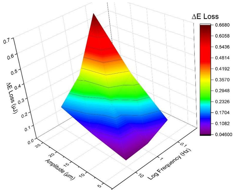
Figure 4:  $\Delta E_{Loss}$  (175°C - 185°C) vs Amplitude and Frequency for HS3
