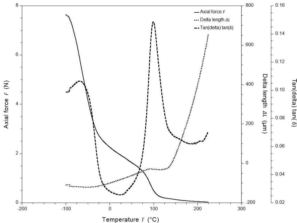
Figure 1: Temperature Ramp @ 1Hz Frequency and 15  $\mu\text{m}$  Amplitude for HS1
