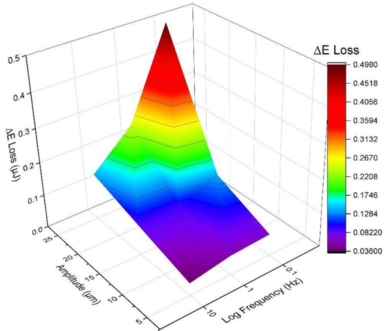
Figure 2:  $\Delta E_{Loss}$  (175°C - 185°C) vs Amplitude and Frequency for HS1
